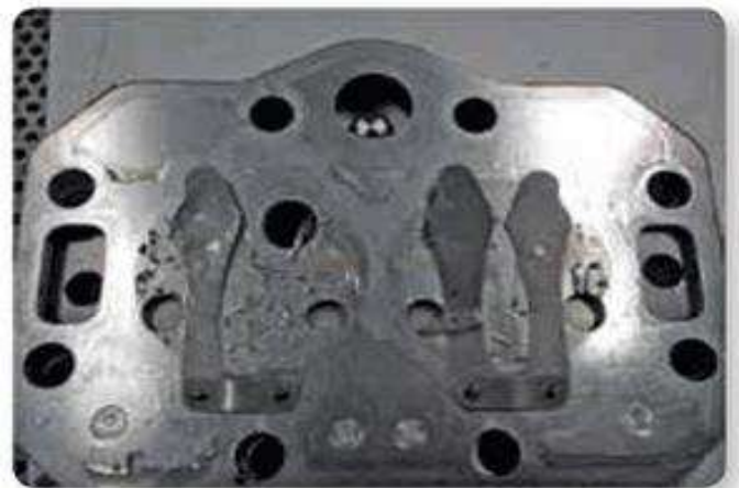
Broken suction reed (liquid slugging).
